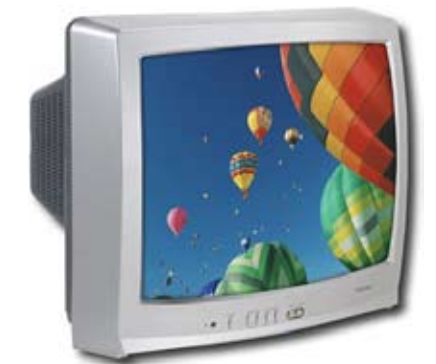
Analog TVs like this one can't use a digital signal without a set-top converter.
